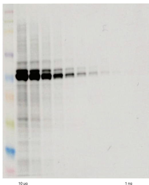
Fig 7. The chemiluminescence mode allows simultaneous imaging of chemiluminescent signals and a colored molecular weight marker. The overlay functionality provides a fast and easy way to verify the molecular weight of detected bands, and identification of band of interest if multiple bands are generated. Amersham ECL Prime detection of ERK1/2 in cell lysates from HeLa cells with ImageQuant LAS 500.
